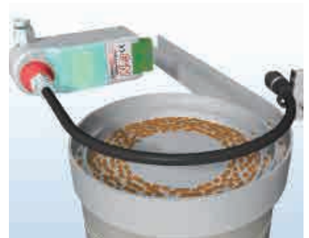
Vibratory bowl feeder (joint nozzle + shower tube)
